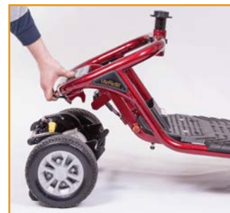
While squeezing the release lever, pull up on the rear frame
